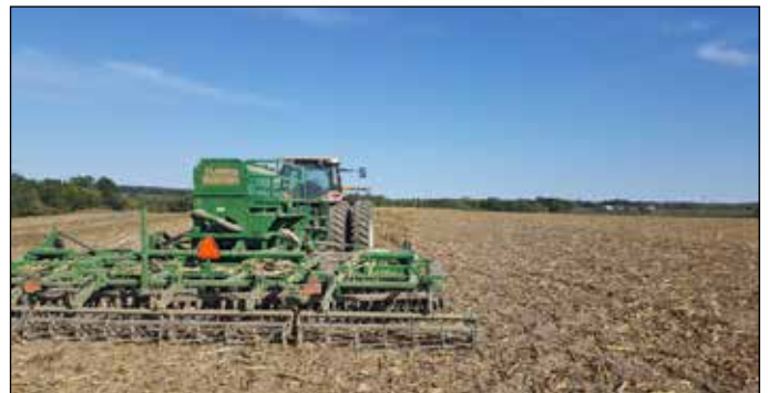
Hodorff’s Turbo Max vertical tillage unit with Turbo Seeder for applying cover crops in one pass after silage harvest
